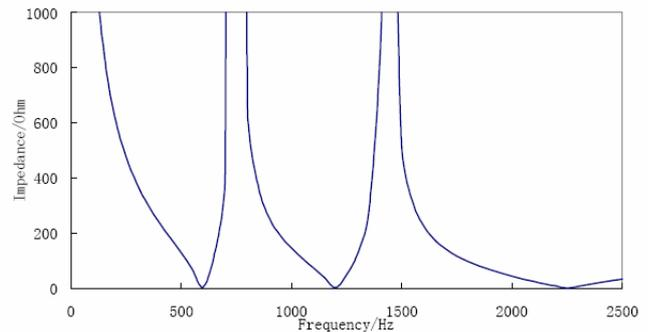
Figure-3: Impedance of DC Filters (TT 12/24/45)
