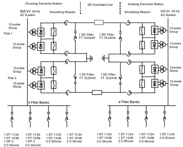
Figure-1: Single Line Diagram of Yun-Guang UHVDC System
