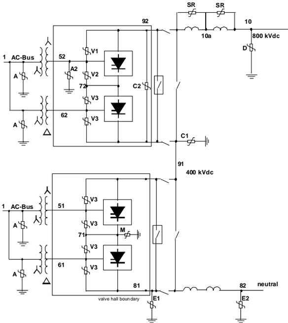
Figure-2: UHVDC Arrester arrangement
