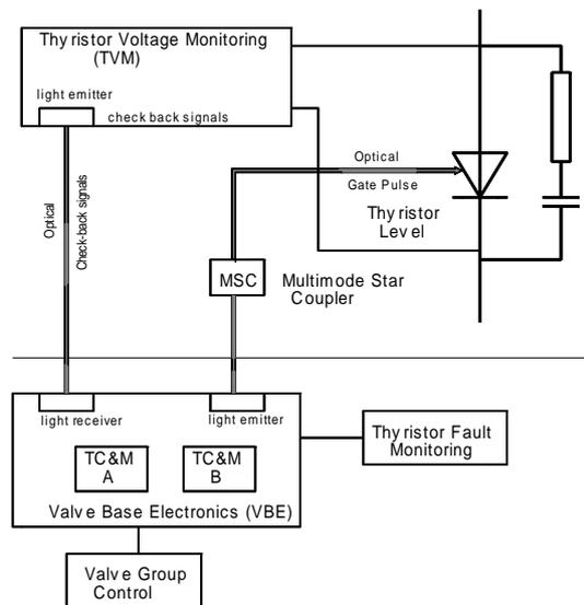
**Figure 4: Block diagram of the valve control for LTT valves**
