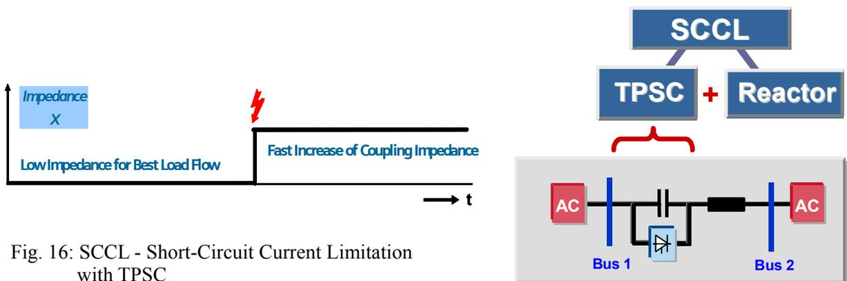
Fig. 16: SCCL - Short-Circuit Current Limitation with TPSC
