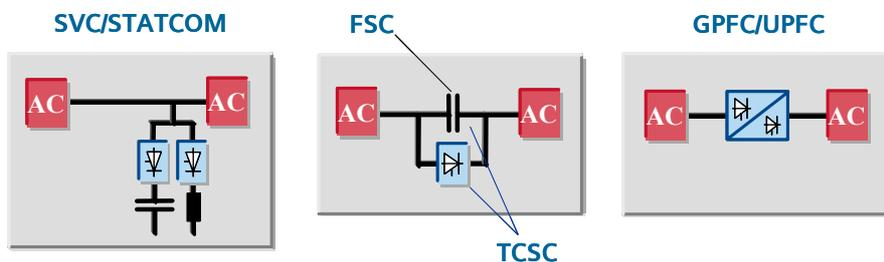
Fig. 4: Basic Configurations of FACTS Devices
