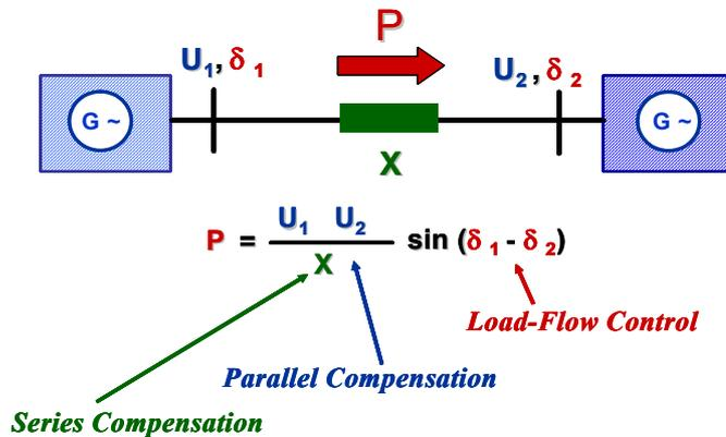
Fig. 3: The Use of FACTS for Power Transmission
