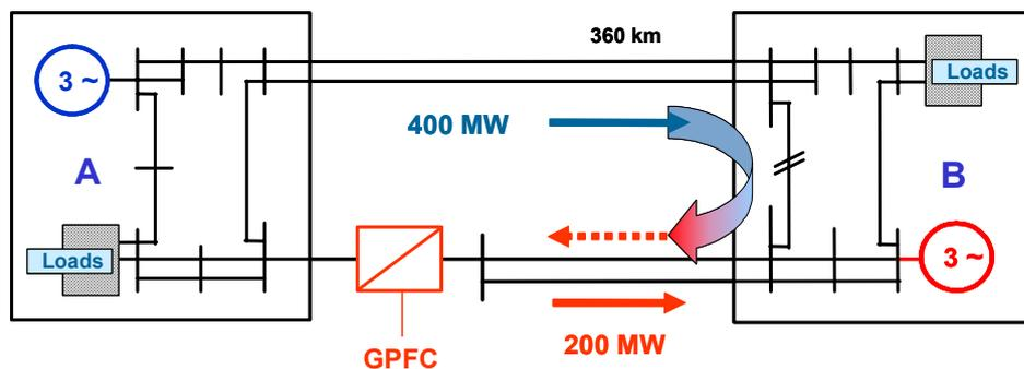
Fig. 8: Avoidance of Loop-Flows with FACTS Grid Power-Flow Controller
