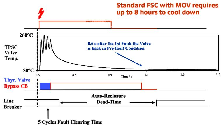
Fig 15: Fast Cooling- Down Time of the High Power Thyristor
