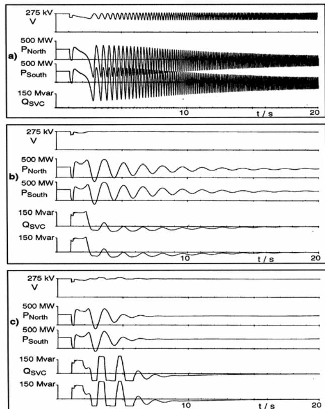
In the recordings in Fig. 12 a), no SVC at the critical node in Harker is connected, the system gets unstable after fault application. In Fig 12 b), both SVC are in voltage control mode, the system already achieves stability and in power oscillation damping mode Fig. 12 c), the damping is significantly improved.
