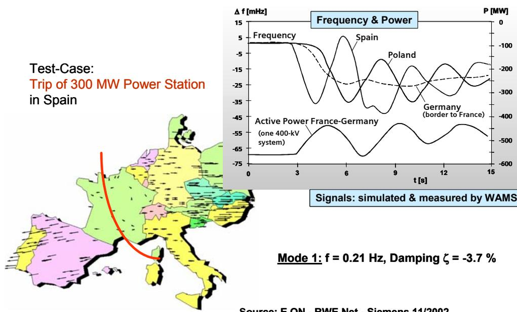
Fig. 10: Interarea-Oscillations in UCTE
