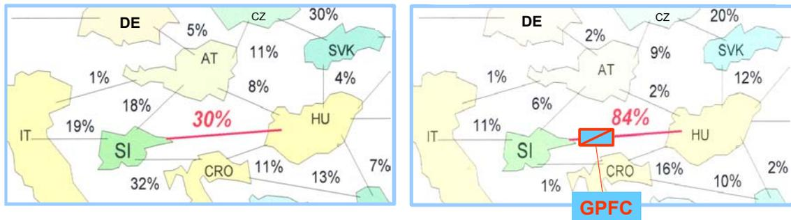
Fig. 9: UCTE – Load-Flow Improvement by means of FACTS
