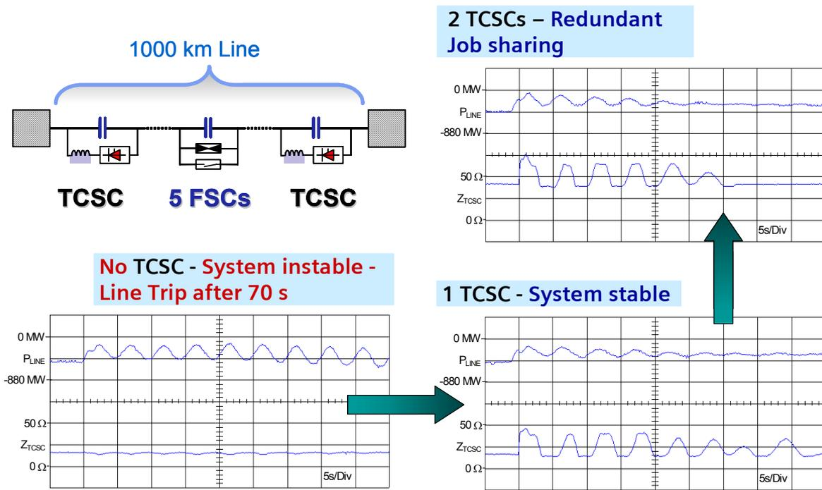
Fig. 11: 500 kV Long Distance AC Transmission in Brazil (Staged-Fault Tests)
