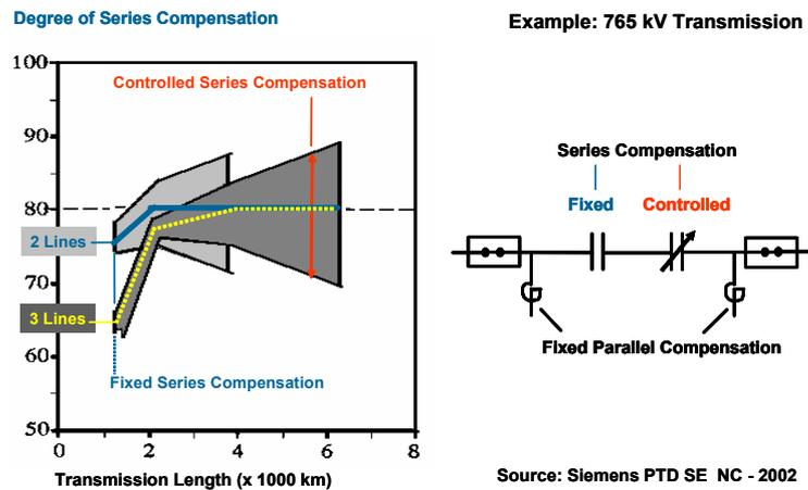
Fig. 7: Limits of long distance AC transmission
