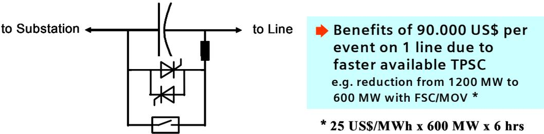
Fig. 13: Operating Principle of TPSC and Cost-Savings for each System Fault
