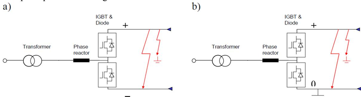
**Figure 3.1:** Grounding of the DC circuit at the Modular Multilevel Converter Stations
