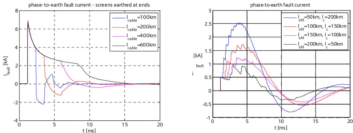
a) Short-circuit current in case of a earthed cable shield, exemplary
