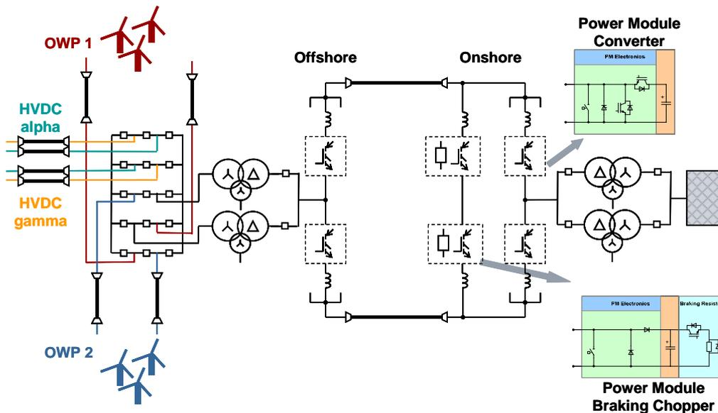
Fig. 2 Overview of HVDC transmission scheme with AC connections to offshore windfarms and adjacent HVDC stations. The number of outgoing AC interconnecting cables varies for various projects due to number of OWP and adjacent HVDC stations.
