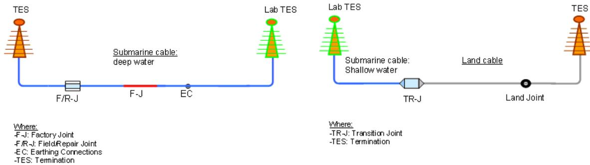
Fig. 8 Loop 1 Testing loops for DC cables.
