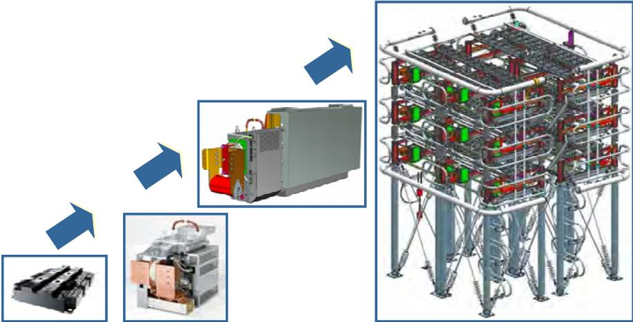
Fig. 3 Construction of HVDC PLUS converter towers from individual power modules.
