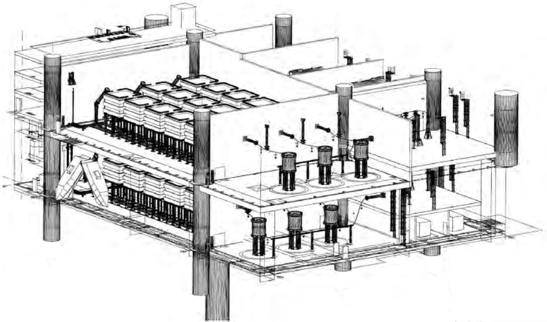
Fig. 4 Crossectional view of offshore platform BorWin2 with HV equipment.
