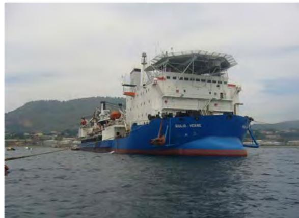
Fig. 9 Cable laying ship Giulio Verne.
