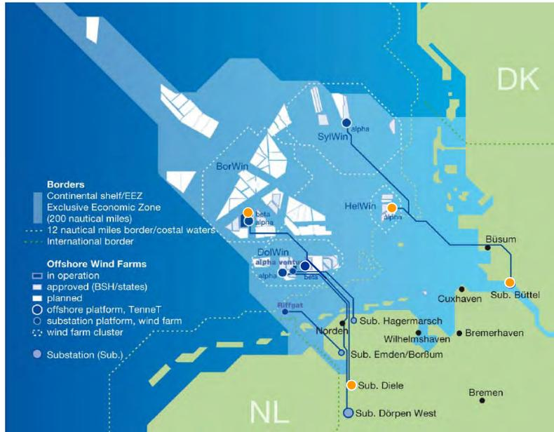
Fig. 1 Location of BorWin2 and HelWin1 projects (stations marked in yellow) together with further windfarm interconnectors.
