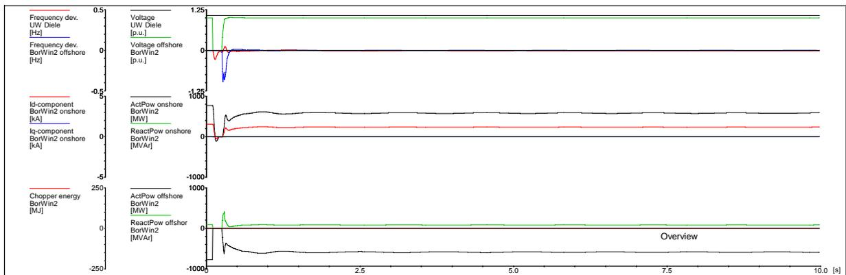
Fig. 10 Offshore 3-phase fault on one export cable of OWP Global Tech 1 feeding BorWin2.
